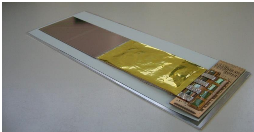
Fig. 4.4.3: Full Silicon strip detector module with FEB-8 connected to the sensor.
