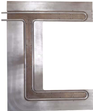
Fig. 4.5.2: Prototype of the heat exchanger for the 1 st Station. Aluminum pipe with a diameter of 8 mm is glued into grooves in the aluminum plate.
