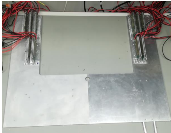
Fig. 4.5.7: Photograph of the test bench for the TIMs. One half of the heat exchanger (left) was machined by a waterjet, while the right part was polished. Thermal contacts of both parts were compared.
