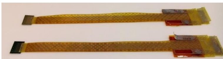
Fig.4.6.13a: ASICs with top and bottom layer micro-cables
