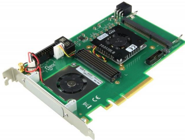
Fig. 4.4.8: TRENZ TEC0330-4 PCIe Gen2 Interface Board as best candidate for the physical interface to the computing node.
