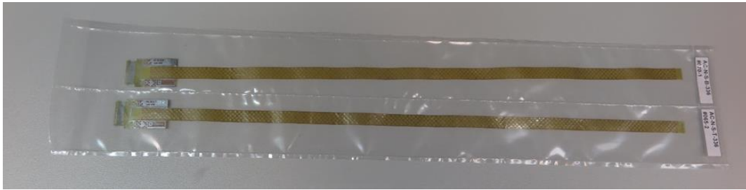
Fig. 4.6.6: Al micro-cables with step test zones in the transport package
