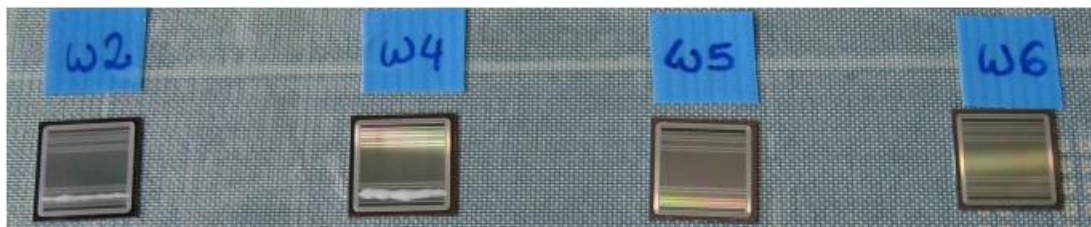
Fig. 4.6.23: prepared small sensors for irradiation test.
