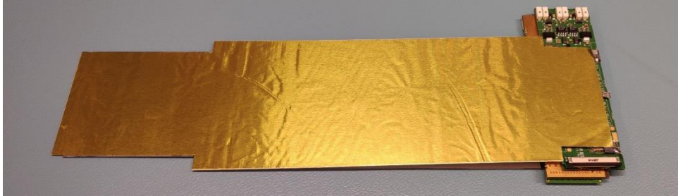
Fig. 4.2.16: Assembled STS module with shielding
